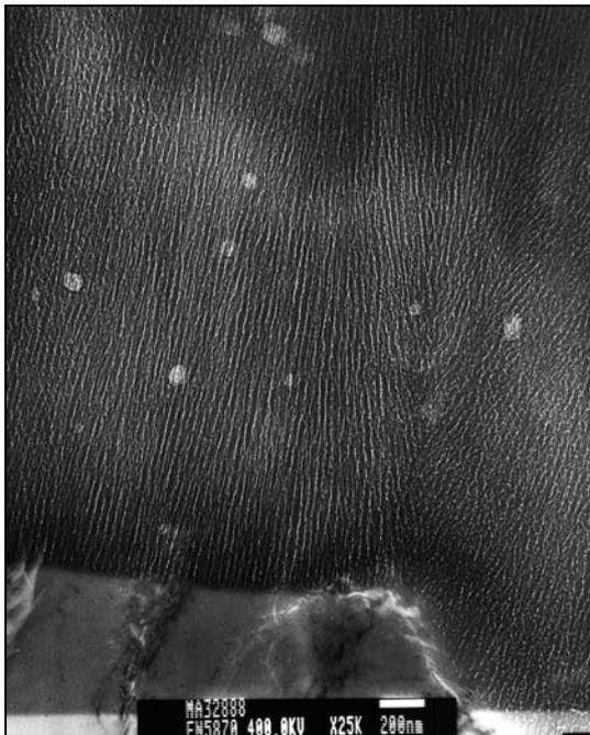
Figure No. 4: Representative TEM micrograph of a Type II anodic oxide finish.
