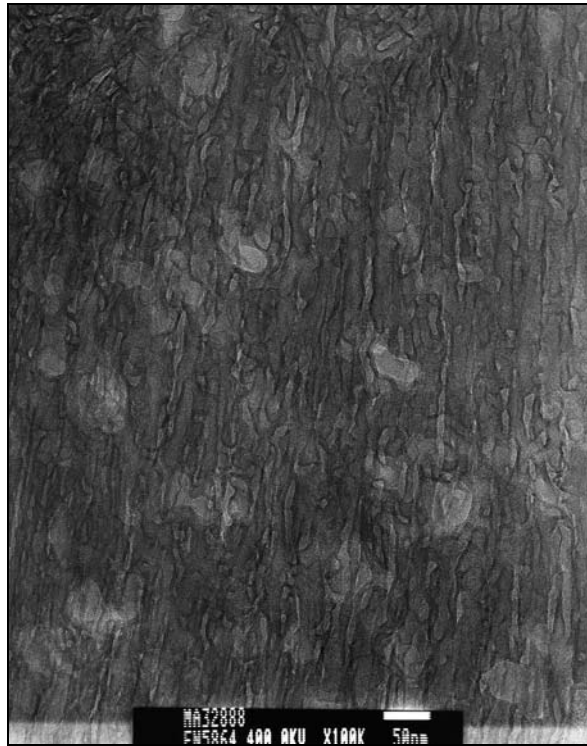
Figure 7: Representative TEM photomicrograph of the modified structure of a composite anodized film. Note the cellular, rather than directly columnar structure.
