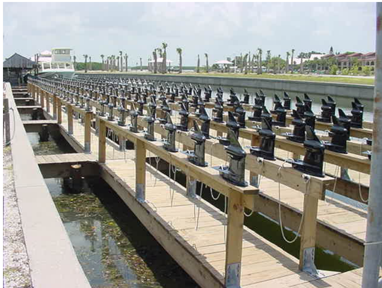
Figure No. 4: Documentary photograph of gear cases with several different types of coating systems being tested in the tidal range of the ocean. Test duration is typically 1 year. The composite samples have been in test for over 6 months.
