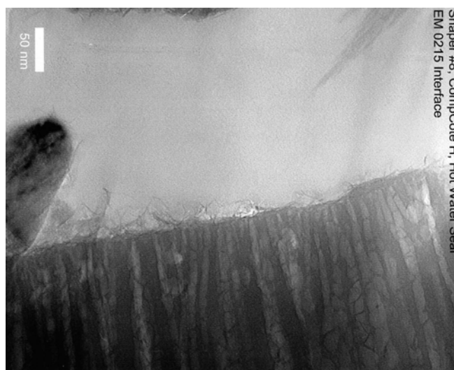
Figure No. 9: TEM image of the interface between the surface of a composite finish processed by way of Type III anodizing parameters and treated with a bonding agent then over-molded with rubber and vulcanized exhibited fibrils extending from the surface of the finish into the polymer layer. EELS analysis of the fibrils determined they were indeed carbon based. No other anodic oxides treated in the same way exhibited these fibrils.
