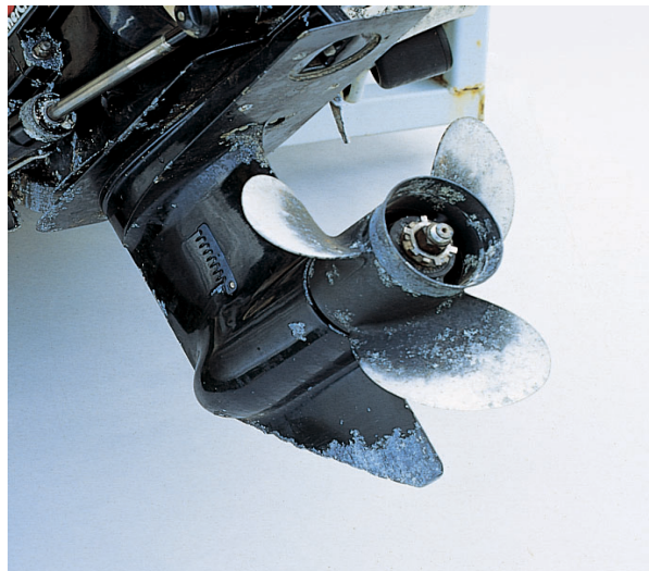
Figure 2: In-field corrosion of outboard engines on the mid- and lower sections of each motor. Note the corrosion initiates and spreads in localized spots. The base and propeller show signs of abrasive wear.
