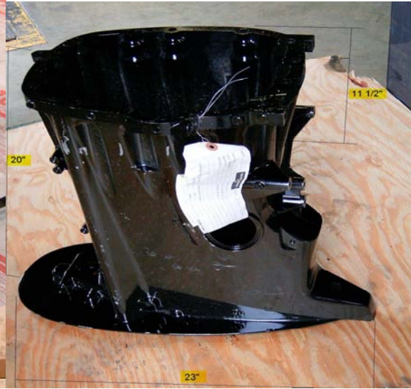
Figure 3: 16 Cylinder head (left). Note the extreme complexity of the part with many small channels and through holes. Not only would the part be anodized, it would also have to be electrodeposition primed. Finish lacquered drive shaft housing (below). The engine components are not only large, they are also heavy.
